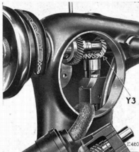
FIG. 28. BACK VIEW, SHOWING BEVEL GEARS IN ARM OF MACHINE
