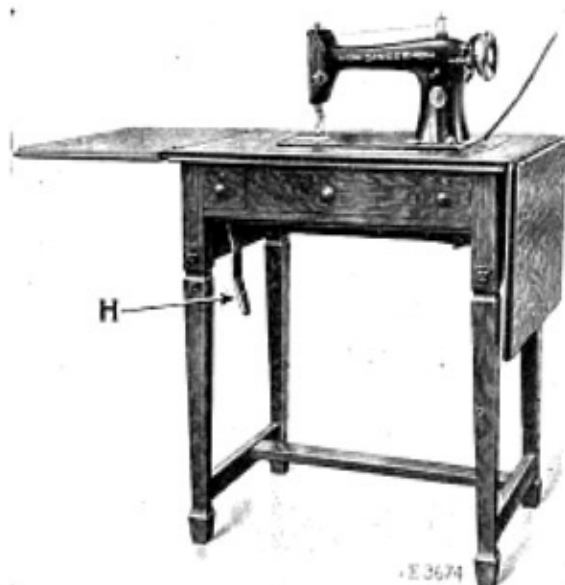
FIG. 32. KNEE LEVER LOWERED INTO POSITION FOR OPERATING
