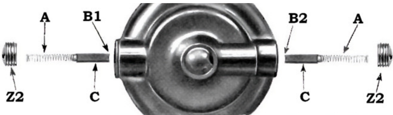
FIG. 25. BRUSHES READY FOR REPLACEMENT (MACHINE 201-3)
