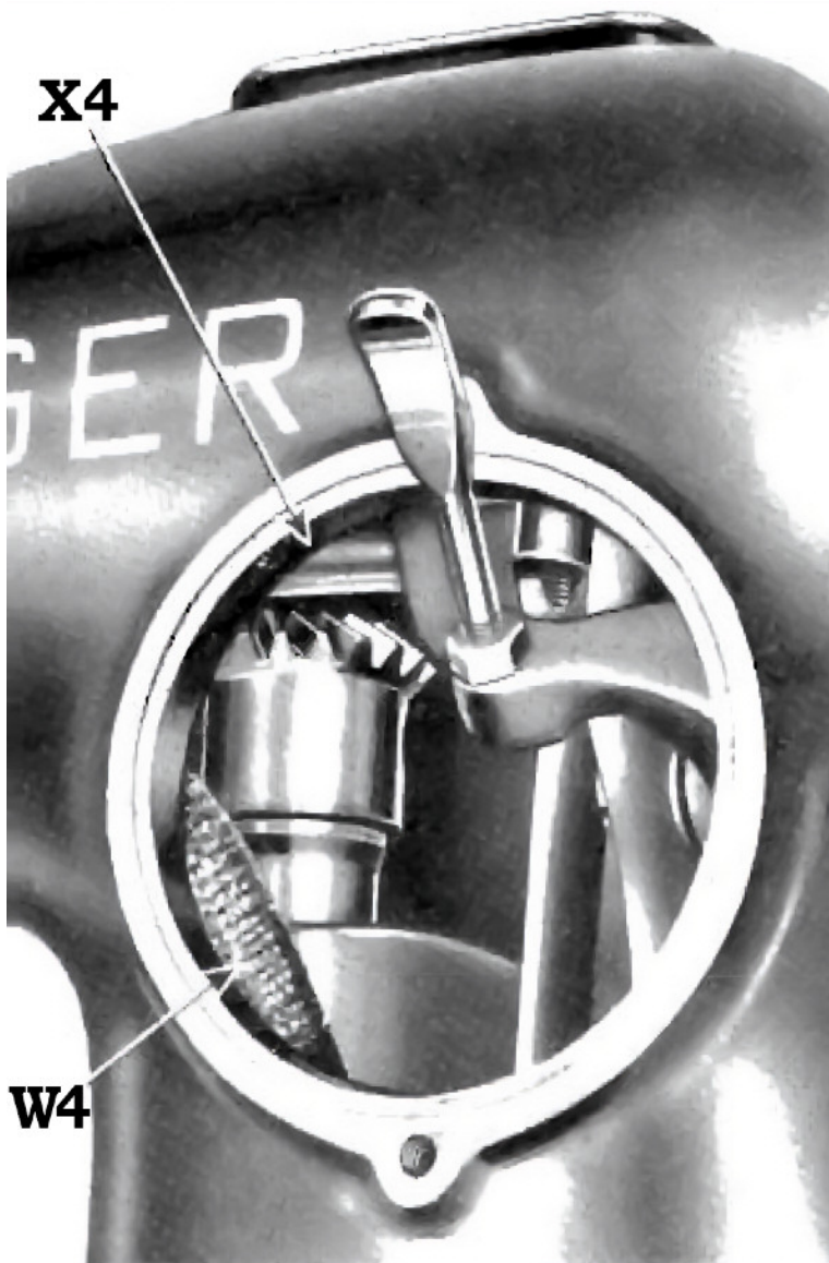
FIG. 11 STITCH INDICATOR PLATE REMOVED TO SHOW THE POSITION OF SINGERLIGHT LEADS IN THE ARM OF MACHINE 201-2
