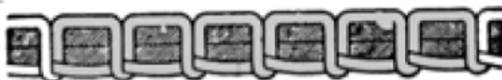
FIG. 13. LOOSE NEEDLE THREAD TENSION
