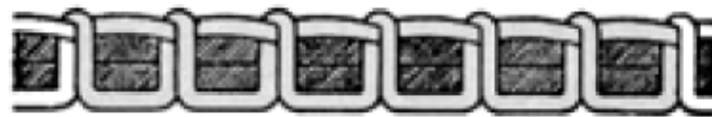
FIG. 12. TIGHT NEEDLE THREAD TENSION
