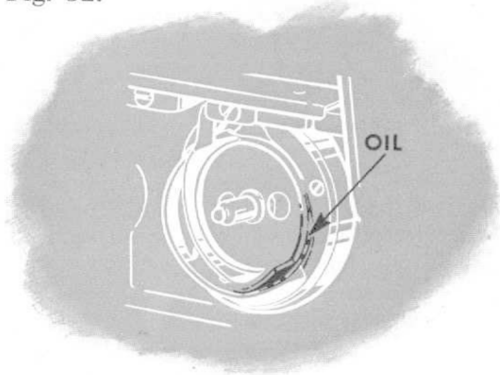
Fig. 32. Oiling Point in Sewing Hook
