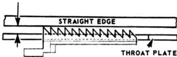
Fig. 25. Feed Dog at Correct Height
